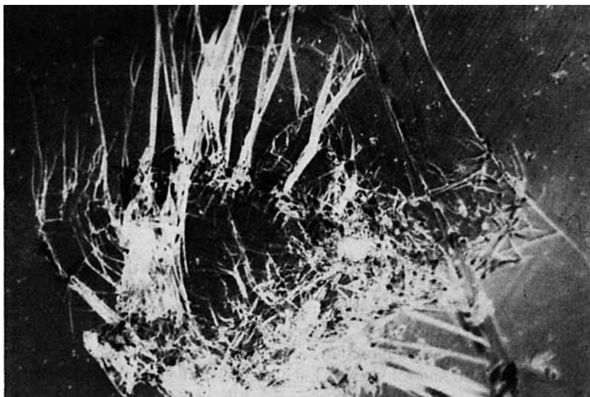
Fig. 2. A damaged area of a titanium trichloride crystal. Optical photomicrograph. 350x.
