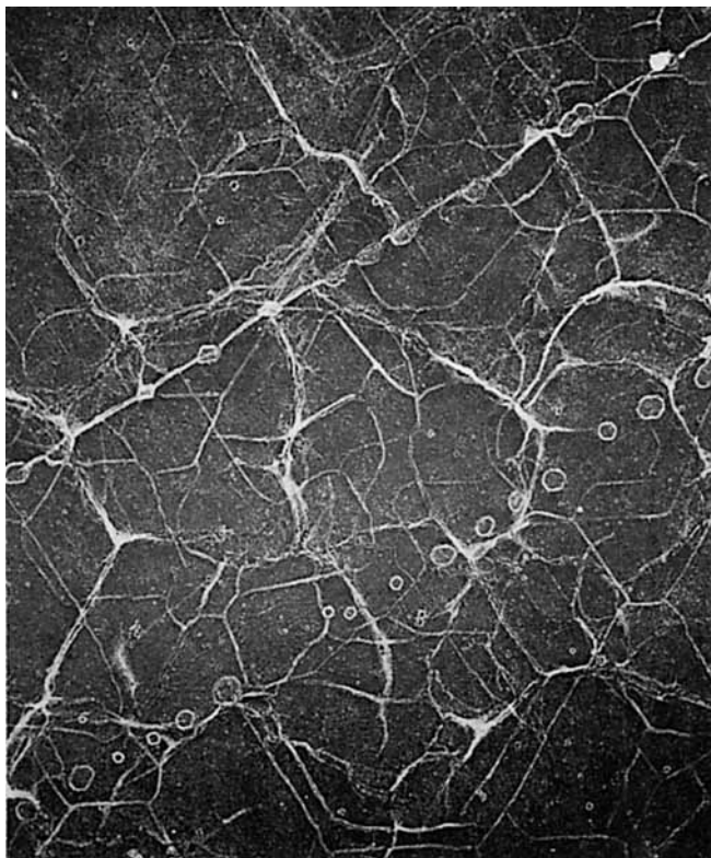
Fig. 9. Electron photomicrograph obtained after only a small amount of polymer had formed. 5200x.
